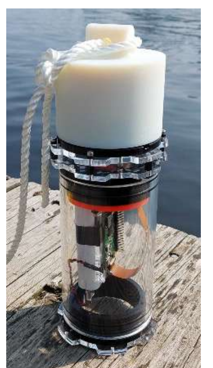
Fig 4. Prototype of underwater digital holographic microscope
