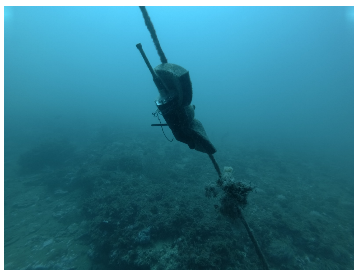
Figure 2 – Hydrophone deployed for data acquisition in southern Portugal, in a rocky reef area located at a depth of approximately 13 m.
