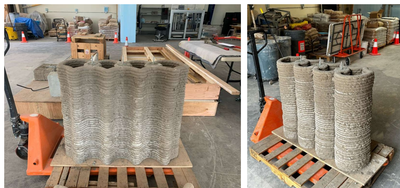
Printed earth wall and columns with threaded steel rods, first post tensioning trials
