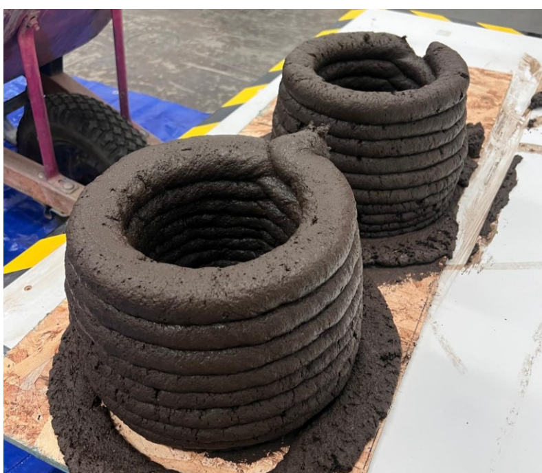
First robotic extrusion trials with the Programmable Mud mix [2].
