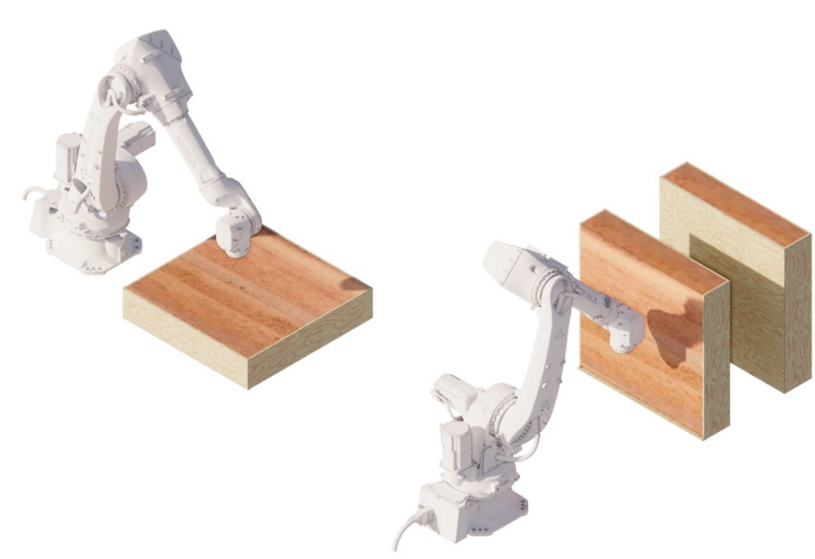
Printing flat avoids the self weight deformation of tall vertical prints
