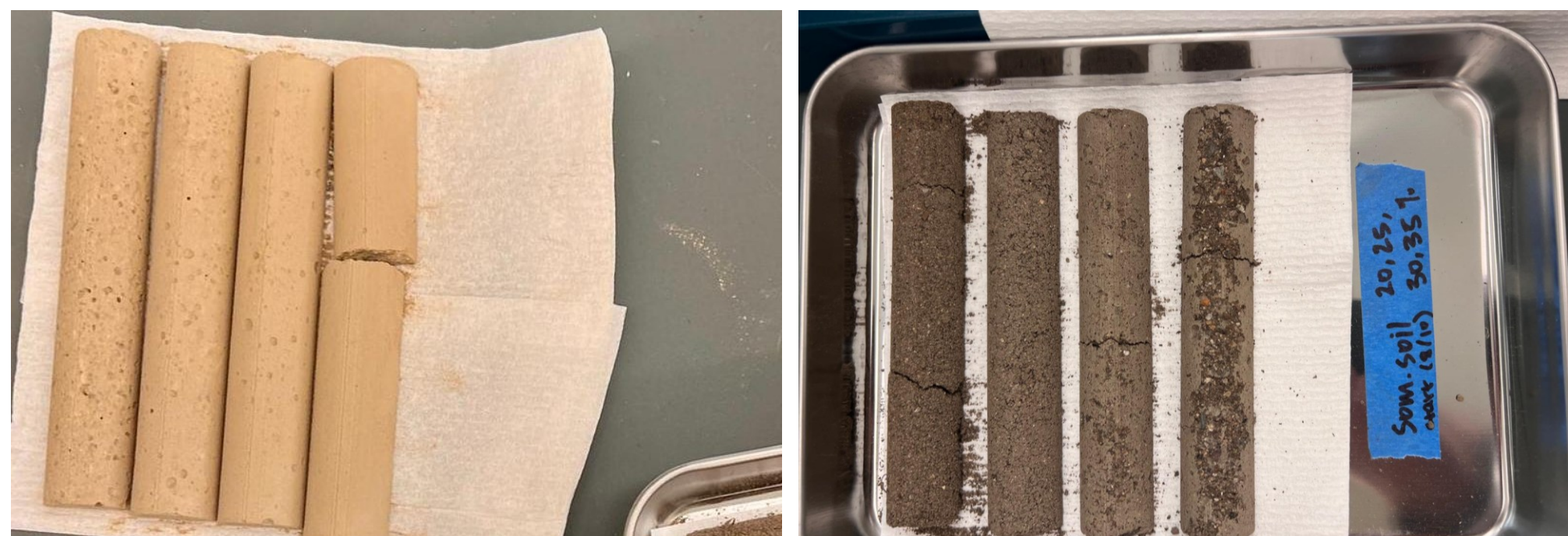
Drying shrinkage bars for two soils, following the protocol in [2].
