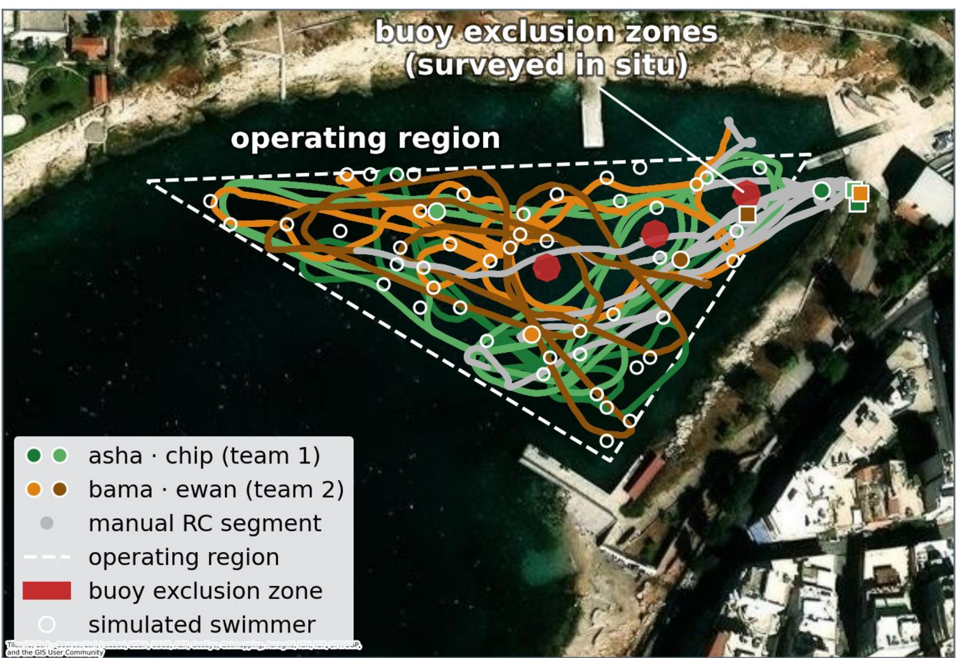
Fig. 4 — Championship rescue heat, 26 June: four student back seats run concurrently inside the shared region, avoiding buoy exclusion zones (red) surveyed in situ.
